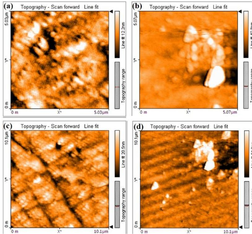
**Fig 4: AFM images depicting surface roughness in(a) untempered chocolate (5x5 μm) (b) tempered chocolate (5x5 μm) (c) untempered chocolate (10x10 μm)(d) tempered chocolate (10x10 μm).**
