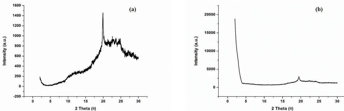
**Fig 3: X-ray diffractogram of (a) untempered chocolate.(b) tempered chocolate.**
